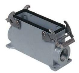
Surface mounting housing, JEI®-V series, with 2 levers, Pg21 x 2 cable entry, size "57.27", high construction
