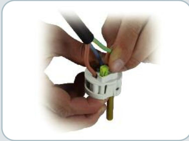
It is in fact sufficient to press the actuator button (pin) to close the spring device of the corresponding terminal, which is supplied open to customers.
