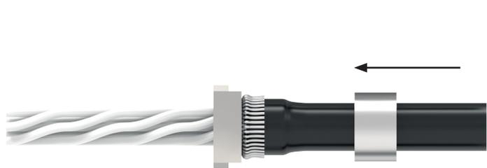
Feed the conductor bundle through the **crimp flange**, pushing it completely underneath the braided shield, then slide the **crimp sleeve** forward over the **flange**.
