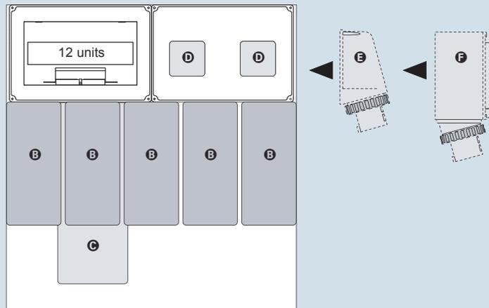
Diagram of the SQV/SQE/SQT devices to be assembled in the empty QG V board
