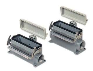
Surface mounting housing, V-TYPE series, with 1 lever, M32 x 2 cable entry, size "104.27", high construction, with plastic cover
