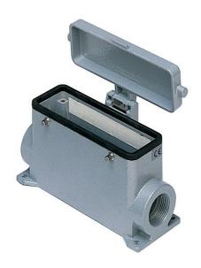
Surface mounting housing, 830V series, with 4 pegs, M32 cable entry, size "104.27", high construction, with metal cover
