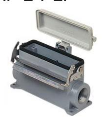
Surface mounting housing, V-TYPE series, with 1 lever, Pg21 cable entry, size "104.27", high construction, with plastic cover
