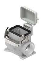
Surface mounting housing, V-TYPE series, with 1 lever, Pg29 x 2 cable entry, size "44.27", high construction, with plastic cover
