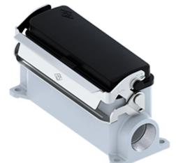
Surface mounting housing, V-TYPE series, with 1 lever, Pg21 cable entry, size "104.27", high construction, with SIMPLEX self-closing cover
