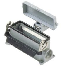
Surface mounting housing, 830V series, with 1 lever, M32 x 2 cable entry, size "104.27", high construction, with metal cover
