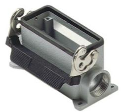
Surface mounting housing, 830V series, with 1 lever, M40 cable entry, size "77.27", high construction
