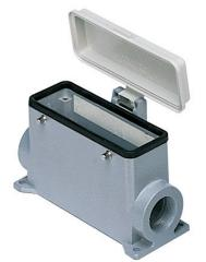
Surface mounting housing, 830V series, with 4 pegs, Pg29 cable entry, size "104.27", high construction, with plastic cover
