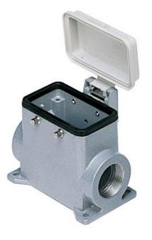
Surface mounting housing, 830V series, with 4 pegs, M32 x 2 cable entry, size "57.27", high construction, with plastic cover
