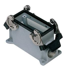
Surface mounting housing, 830V series, with 2 levers, M40 cable entry, size "57.27", high construction
