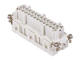
Female insert, JSE series, spring terminal connection, 24 poles + PE (25-48), 16 A 500 V 6 kV 3, size "104.62"
