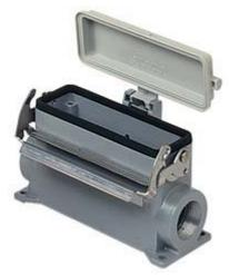
Surface mounting housing, JEI®-V series, with 1 lever, M32 x 2 cable entry, size "57.27", high construction, with plastic cover
