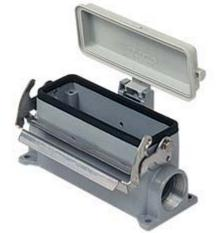
Surface mounting housing, JEI®-V series, with 1 lever, Pg21 x 2 cable entry, size "104.27", with plastic cover
