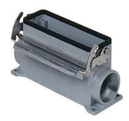
Surface mounting housing, JEI®-V series, with 1 lever, Pg21 x 2 cable entry, size "57.27", high construction
