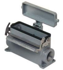
Surface mounting housing, V-TYPE series, with 1 lever, Pg29 x 2 cable entry, size "77.27", high construction, with metal cover
