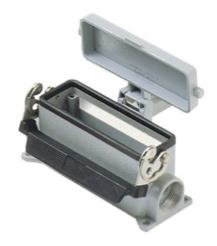
Surface mounting housing, 830V series, with 1 lever, Pg21 x 2 cable entry, size "104.27", with metal cover
