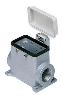
Surface mounting housing, 830V series, with 4 pegs, Pg21 cable entry, size "57.27", high construction, with plastic cover
