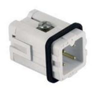
Male insert, JKS series, spring terminal connection, 3 poles + PE, 10 A 400 V 4 kV 3, size "21.21"
