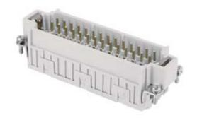
Male insert, JDS series, spring terminal connection, 42 poles + PE (43-84), 10 A 400 V 6 kV 3, size "104.62"
