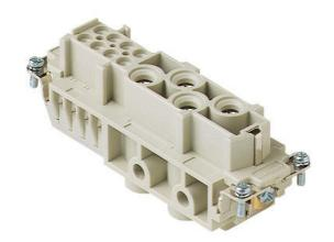
Female insert, CX series, screw terminal connection, 4 + 8 poles + PE, 80 A 400 V 6 kV 3 / 16 A 230/400 V 4 kV 3, size "104.27", without plate
