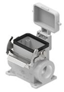
Surface mounting housing, V-TYPE series, with 1 lever, Pg21 cable entry, size "44.27", high construction, with metal cover
