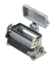
Surface mounting housing, 830V series, with 1 lever, Pg29 cable entry, size "77.27", high construction, with metal cover
