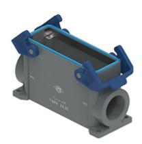
Surface mounting housing, T-TYPE /H series, with 2 levers, M40 cable entry, size "104.27", with integrated protective PE jumpers
