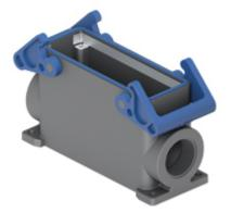
Surface mounting housing, T-TYPE/C series, with 2 levers, M40 cable entry, size "104.27", with integrated protective PE jumpers
