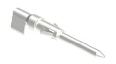
Male crimp contact, SD series, 10 A, stamped silver plated, wire cross section 1,5 - 2,5 mm<sup>2</sup>, AWG 16 - 14, loose parts, for 500 mating cycles
