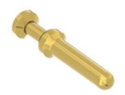
Male crimp contact, RX series, 40 A, turned gold plated, wire cross section 10 mm<sup>2</sup>, AWG 8, HNM - High Number of Matings version
