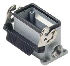
Surface mounting housing, 830V series, with 1 lever, M20 x 2 cable entry, size "57.27"
