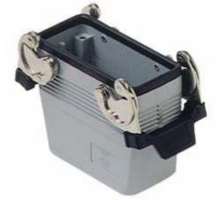
Hood, 830V series, with 2 levers, M25 top cable entry without adapter, size "104.27", high construction
