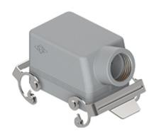
Hood, C-TYPE series, with 2 levers, M32 side cable entry, size "66.40", without gasket
