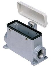
Surface mounting housing, C-TYPE series, with 4 pegs, M32 x 2 cable entry, size "104.27", high construction, with plastic cover
