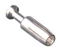
Female crimp contact, CX series, 40 A, turned silver plated, wire cross section  $10\ mm^2$ , AWG 8, cable diameter up to 7,5 mm
