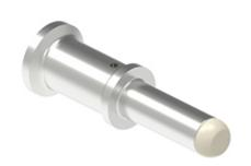
Male crimp contact, CX7 series, 70 A, turned silver plated, wire cross section 25 mm<sup>2</sup>, AWG 4 - 3, finger-proof version
