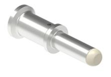
Male crimp contact, CX7 series, 70 A, turned silver plated, wire cross section 10 mm<sup>2</sup>, AWG 8 - 7, finger-proof version
