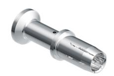
Female crimp contact, CX7 series, 70 A, silver plated, wire cross section 6 mm², AWG 10
