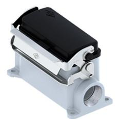
Surface mounting housing, V-TYPE series, with 1 lever, Pg21 cable entry, size "77.27", high construction, with SIMPLEX self-closing cover
