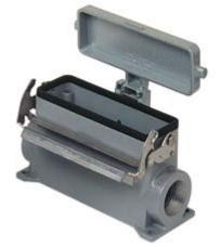
Surface mounting housing, V-TYPE series, with 1 lever, Pg29 cable entry, size "77.27", high construction, with metal cover
