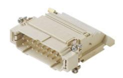
Male insert, CT series, screw terminal connection, 16 poles + PE, 16 A 230/400 V 4 kV 2, size "77.27", with incorporated terminal block, right side mounting
