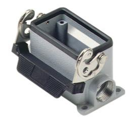
Surface mounting housing, 830V series, with 1 lever, Pg16 cable entry, size "57.27"
