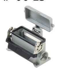
Surface mounting housing, 830V series, with 1 lever, Pg21 cable entry, size "77.27", high construction, with metal cover
