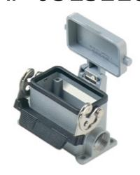
Surface mounting housing, 830V series, with 1 lever, Pg29 x 2 cable entry, size "57.27", high construction, with metal cover
