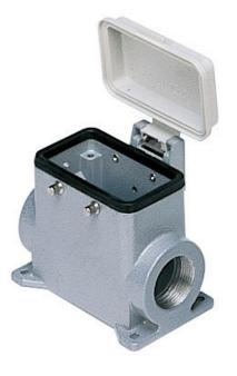
Surface mounting housing, 830V series, with 4 pegs, Pg29 x 2 cable entry, size "57.27", high construction, with plastic cover
