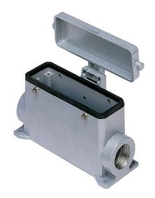
Surface mounting housing, C-TYPE series, with 4 pegs, Pg21 cable entry, size "104.27", with metal cover
