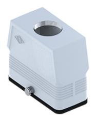
Hood, CENTRAL LEVER series, with 2 pegs, Pg29 top cable entry without adapter, size "77.27", high construction
