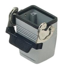
Hood, C-TYPE series, with 1 lever, Pg29 top cable entry without adapter, size "44.27", high construction
