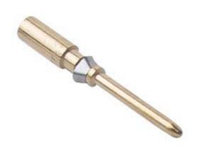
Male crimp contact, CD series, 10 A, turned gold plated, wire cross section 1 mm<sup>2</sup>, AWG 18, high thickness gold plating
