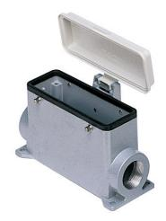
Surface mounting housing, C-TYPE series, with 4 pegs, Pg29 x 2 cable entry, size "104.27", high construction, with plastic cover
